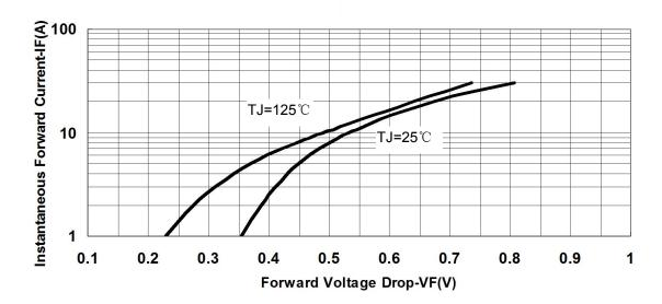
Fig.3-Typical Instantaneous Forward Voltage Characteristics
